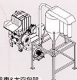
加風車&太空包架 Conveyor feeding
