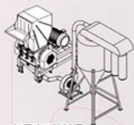
加風車&儲料桶 Blower and temporary storage tank
