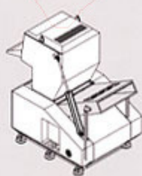
加後槽投入 Feed the scrap from the rear chute
