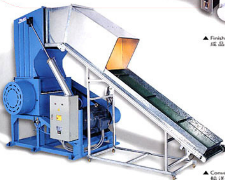
▲ Convey plastic chair to crusher machine 輸送涼椅到粉碎機
