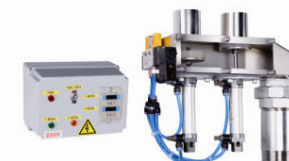
MODEL: AC-38 TUBE DIAMETER : Ø38mm CAPACITY : 200~300kg/hr PRESSED AIR : 4.5kg/cm²G MACHINE SIZE : 330*150*150mm
